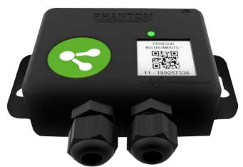
With the General Purpose Phantom you can adapt the data collection to your specific needs. Take **any 2Vpp sensor** and make it wireless.
