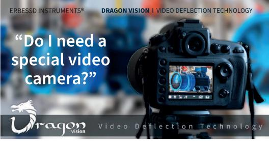
Any camera works for **DragonVision™** although, the better the quality of the recording, the better the results. In fact, tests made with a camera of an iPhone XS with slow motion recordings at 1 meter of distance showed a resolution in amplitude of 0.1 thousandhts of an inch (2.54 microns) and 120 Hz frequency (7,200 CPM). Which is very useful for 95% of common machines.
