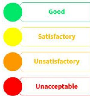
By default, the application takes the **ISO-10816** values and sets the machine as **Class II**. There are 2 default severity alarms, *velocity - CLASS II*, and *acceleration envelope - CLASS II*. **ISO-10816** has 4 machine types and divides the vibration values as follows:
